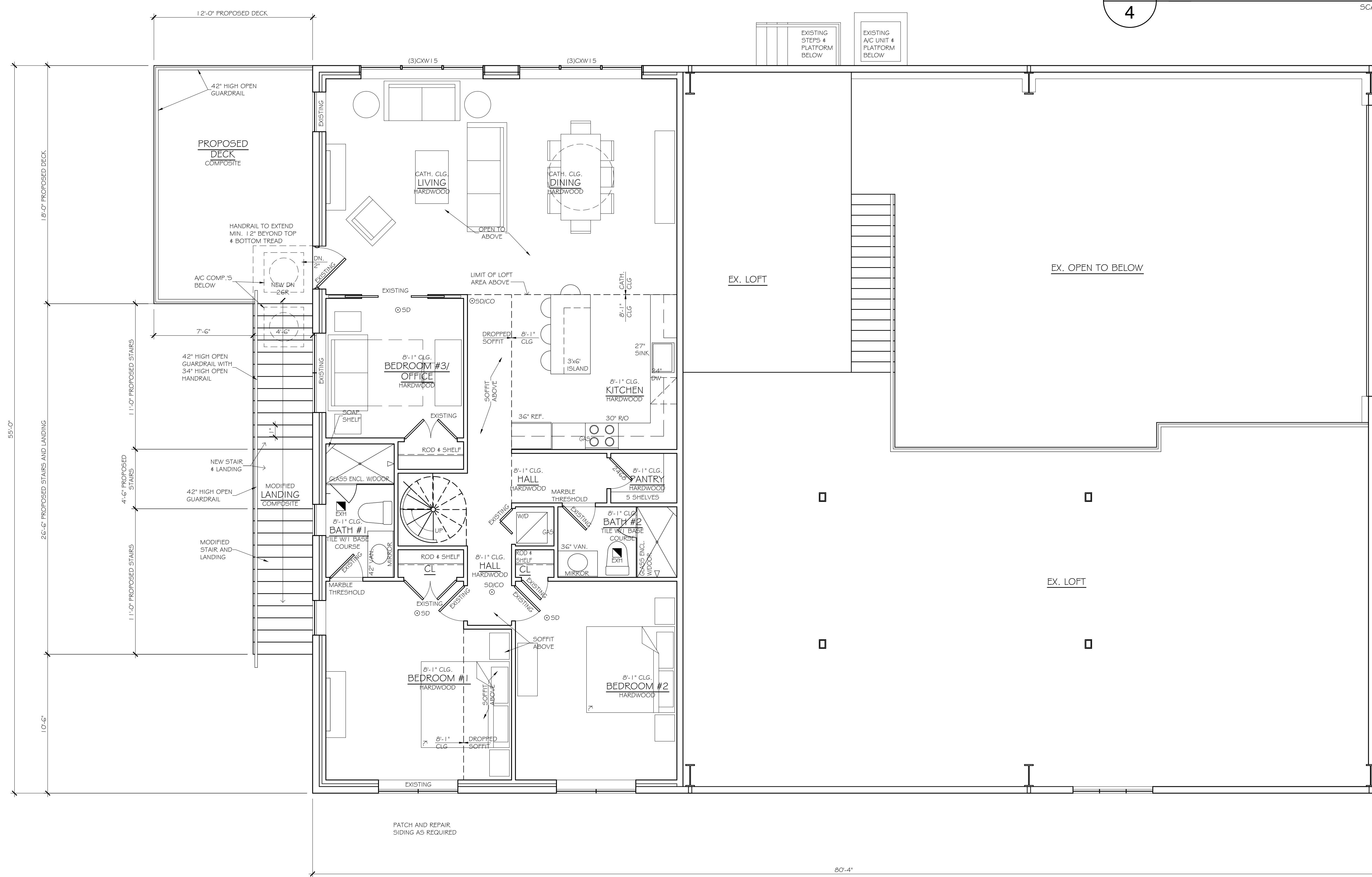
EXISTING SECOND FLOOR PLAN W/PROPOSED DECK SCALE: 1/4" = 1'-0"
